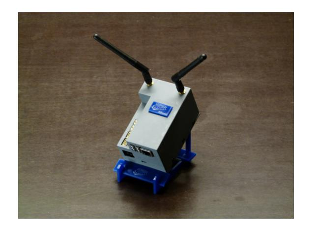
A fast wireless transceiver is integrated which allows the use of ground based sensors in the control loop. Up to five antennas can be connected. Basic driver and control software is included. Client specific software development for competitive costs on request.
